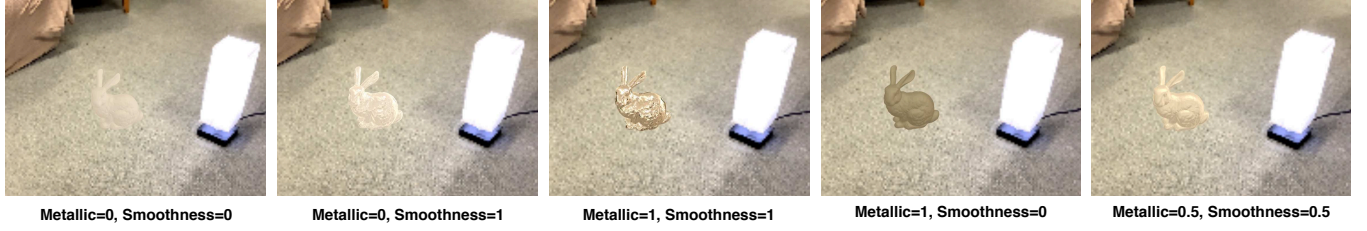
Figure 16: AR scenes rendered with XIHE with different materials. Both metallic and smoothness are Unity parameters.
