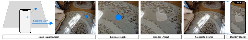
Fig. 2. Lighting estimation workflow in AR applications. Lighting estimation starts from a camera view captured by a user’s mobile phone camera. The captured photo, together with a screen coordinate (e.g., provided by the user through touch-screen), is then passed to a lighting estimation algorithm. The estimated lighting information is then used to render 3D objects, which are then combined with the original camera view into a 2D image frame.
