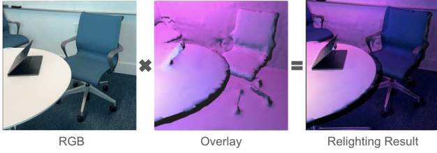
Fig. 3: An example of the mesh quality directly from the LiDAR camera on the iPhone 16 Pro. The errors in such suboptimal mesh can significantly reduce the visual quality of the final relit image, especially around the edges.
