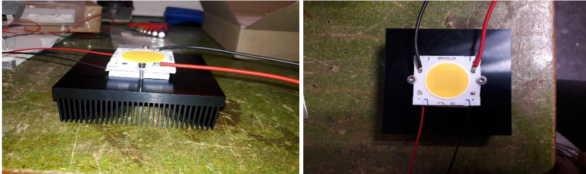
Figure 3: The first prototype LED + TEG1+dissipator
